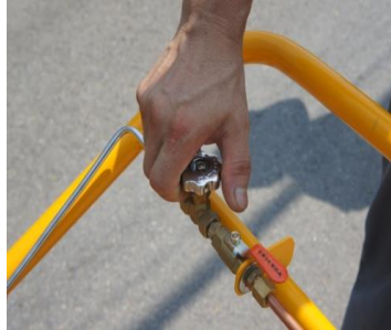
Chemical supply Valve
